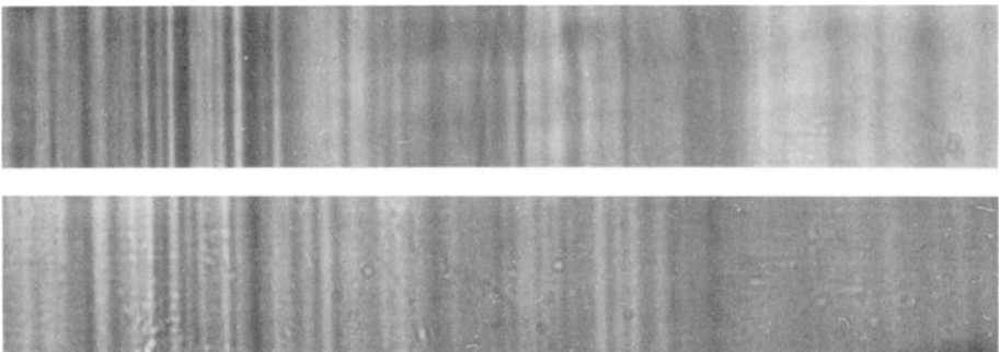
FIG. 6—Comparison of ream marks that are separated by 70 cm.
